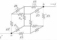
Let current *I* enter at *a* and exit at *b*. At *a* there are three equivalent branches, so current is I/3 in each. At the next junction point there are two equivalent branches so each gets current I/6. Then at *b* there are three equivalent branches with current I/3 in each. The voltage drop from *a* to *b* then is  $V = (\frac{r}{3})R + (\frac{r}{6})R + (\frac{r}{3})R = \frac{5}{6}IR$ . This must be the same as  $V = IR = \frac{5}{6}R$ .
